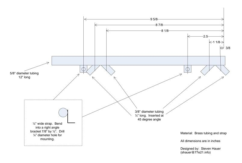
Wiring holder mounts to two rear-most studs on valve cover on exhaust side of engine. 3/8 inch tubes are for mounting 3/8 inch convoluted tubing used for each individual coil connector. Wiring holder is made from brass tubing available at many hobby shops and is soldered together. Shield ground wires from each coil are routed to the front of the holder, all other wires are routed to the rear of the holder.
